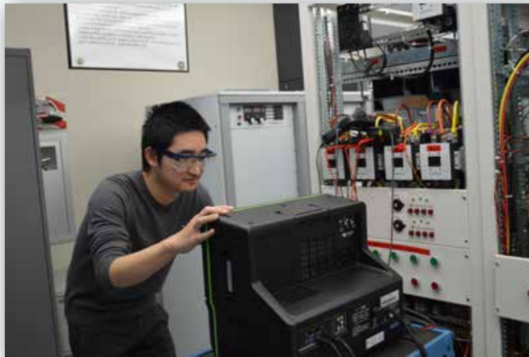
Ph.D. student Yalong Li monitors a multiterminal HVDC hardware testbed.
