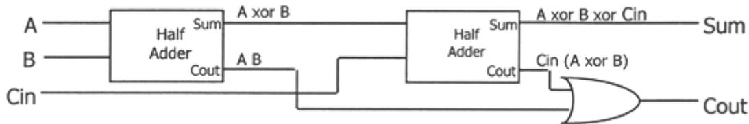
Show how to implement the full adder Sum and Carryout in multilevel form using **NAND gates only**. You may assume that the input variables A, B, Cin and their complements are available. Sketch your solution as a logic schematic (you may only use NAND gates).
