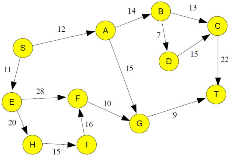
Your job is to perform a maximum flow determination on this graph using a standard augmenting path algorithm. To determine each augmenting path, you must perform a depth-first search on the graph, where you traverse edges in the depth-first search in order from greatest capacity to least capacity. In CS302, we called this the “greedy DFS” path determination.
